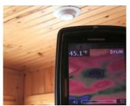
test gives members a great look at where air is infiltrating / escaping. The cooperative's infrared camera can be used to track and photograph temperature differences to highlight hidden points that drive up a home's energy usage.
