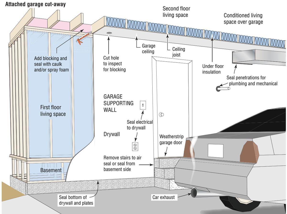
*Air sealing garage penetrations can present a challenge. Easy tasks involve caulking obvious penetrations such as electrical outlets, the drywall perimeter and bottom plates of the foundation. More difficult tasks involve cutting away ceiling drywall in the garage to check for and provide blocking between the garage and the floor system adjacent to the garage.*
