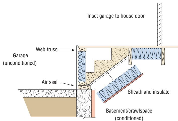
If accessible, seal and block behind the stairs from the garage side if the stairs can be pulled away from the foundation. In some instances, garage stairs can be accessed and air sealed from the inside of the basement or crawlspace. For example, recessed doors from the garage to the living space may require working behind and underneath the stairs. Use rigid foam board and insulation batts to seal and insulate this space.
